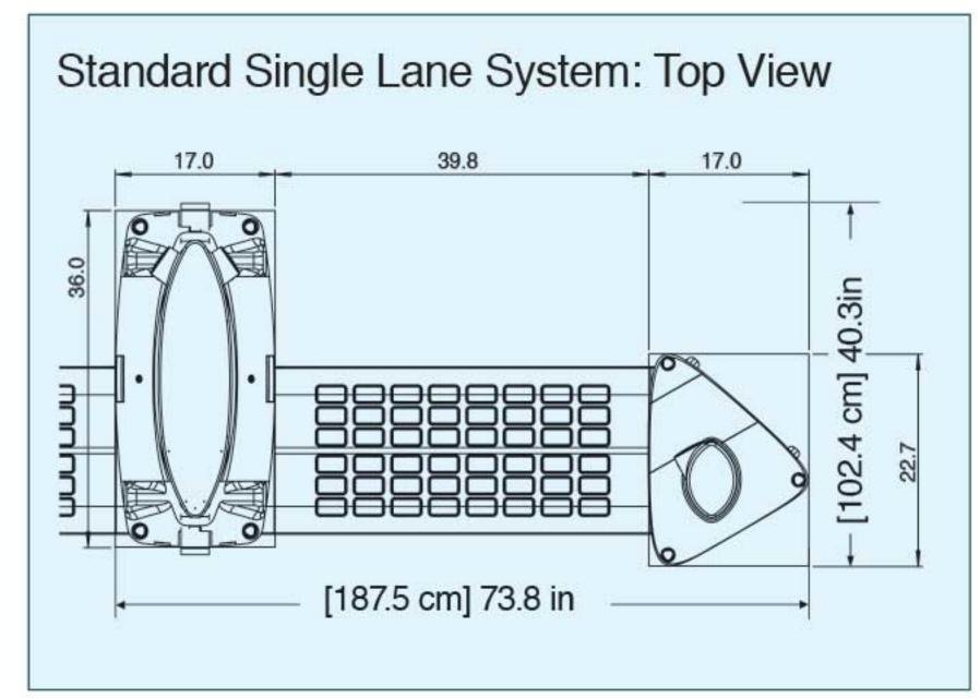
Note: Evolv Express® must not be sprayed with high- or low-pressure water or liquid; doing so could damage the system and will void the warrantyAll dimensions are +/- 1 cm.
